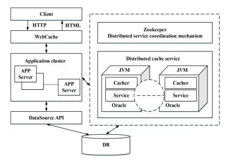
Fig. 1. Distributed cache overall architecture diagram
